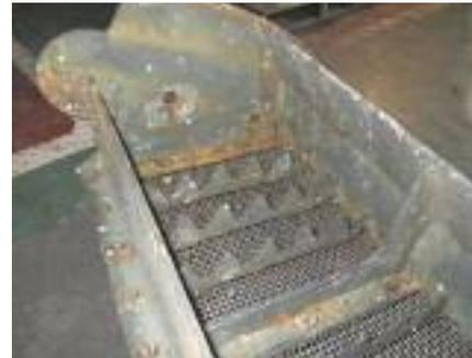
After a recent review it was decided to completely re-coat the screen. Corrocoat Japan completed the work by abrasive blasting the screen then spray applying Polyglass ZipCoat, and a top coat
