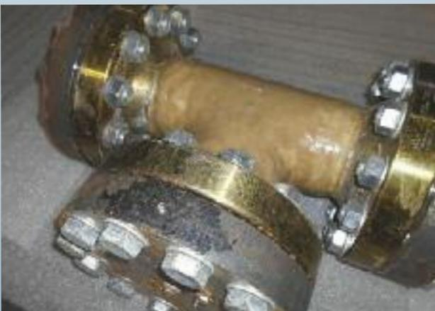
Materials Research Laboratory. The CSR system uses a combination of Corrocoat specialist coatings interlayered with GRP composite laminates to repair, corrosion protect and give structural strength to pipework and other equipment, at a fraction of the cost and inconvenience of replacement. It is an ideal solution for capital process equipment where corrosion has reduced the wall thickness to below an acceptable minimum or where damage has occurred.
