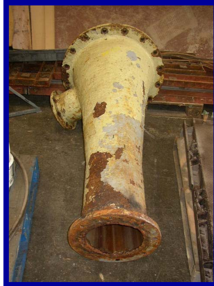
The venturi on arrival in our Leeds works.
