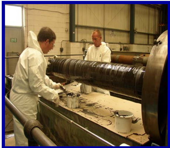
The roller is pre-machined, and grit blasted before the application process begins.
