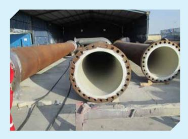
As part of a series of initial projects, a number of pipespools required repair and restoration from corrosion damage at a seawater injection plant. The project ran over 9 months and Polyglass VEF was the primary coating system used throughout. Polyglass VEF was the ideal coating system for this project, protecting the spools from future corrosion damage from seawater and in turn extending their service life considerably.
