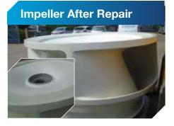
The impeller was then sent back to the Corrocoat workshop to be coated with Corroglass 600.
